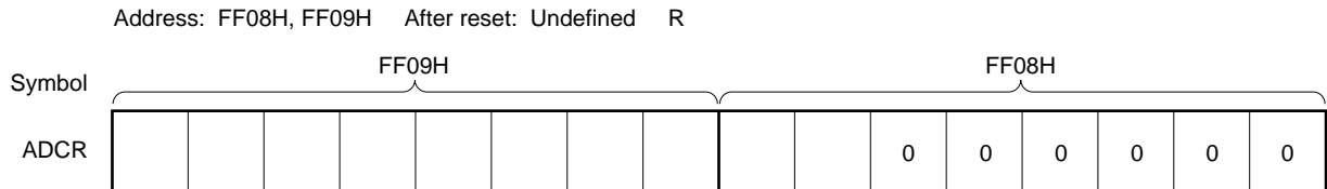
Figure 12-5. Format of A/D Conversion Result Register (ADCR)
